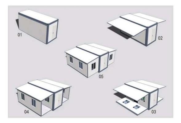
The expandable container house will be finished 90% in the factory, you just need to expand the folded container house.
